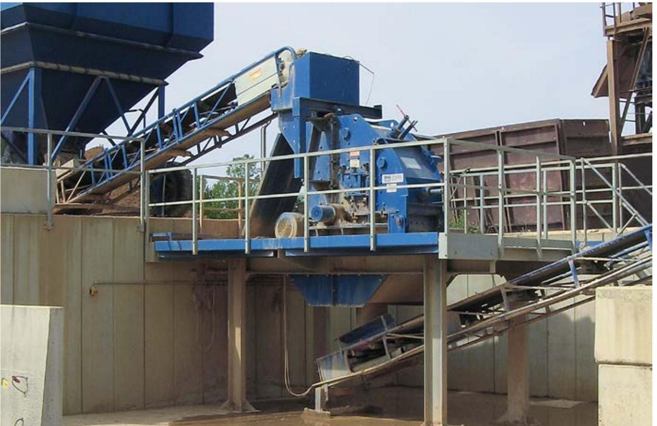
A BHS Impact Crusher of type PB 0806 is used for crushing oversized gravel (32 to 250 mm) to produce saleable chippings.
